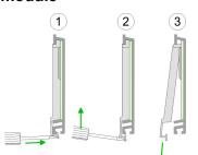
**1.** Dismantle the according protection flaps of the SPEED-Bus slot with a screw driver (open and pull down).
