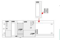
Repeat this procedure with the peripheral modules, by clicking a backplane bus coupler, stick the module right from the modules you've already fixed, click it downwards and connect it with the backplane bus coupler of the last module and bolt it.
