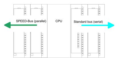
**Serial Standard bus** The single modules are directly installed on a profile rail and connected via the backplane bus coupler. Before installing the modules you have to clip the backplane bus coupler to the module from the backside. The backplane bus couplers are included in the delivery of the peripheral modules.
