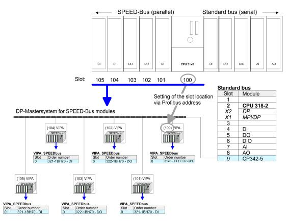
The according module is to be taken over from the HW Catalog of vipa\_speedbus to slot 0.
